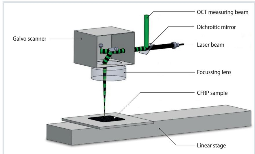
**Fig. 1.** The setup combines laser material processing with an optical measurement technique to automate the laser process Source: LZH, graphic: © Hanser
