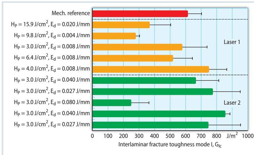
**Fig. 3.** Depiction of interlaminar fracture toughness realized by two near-infrared laser sources in comparison to mechanically milled references Source: LZH, graphic: © Hanser
