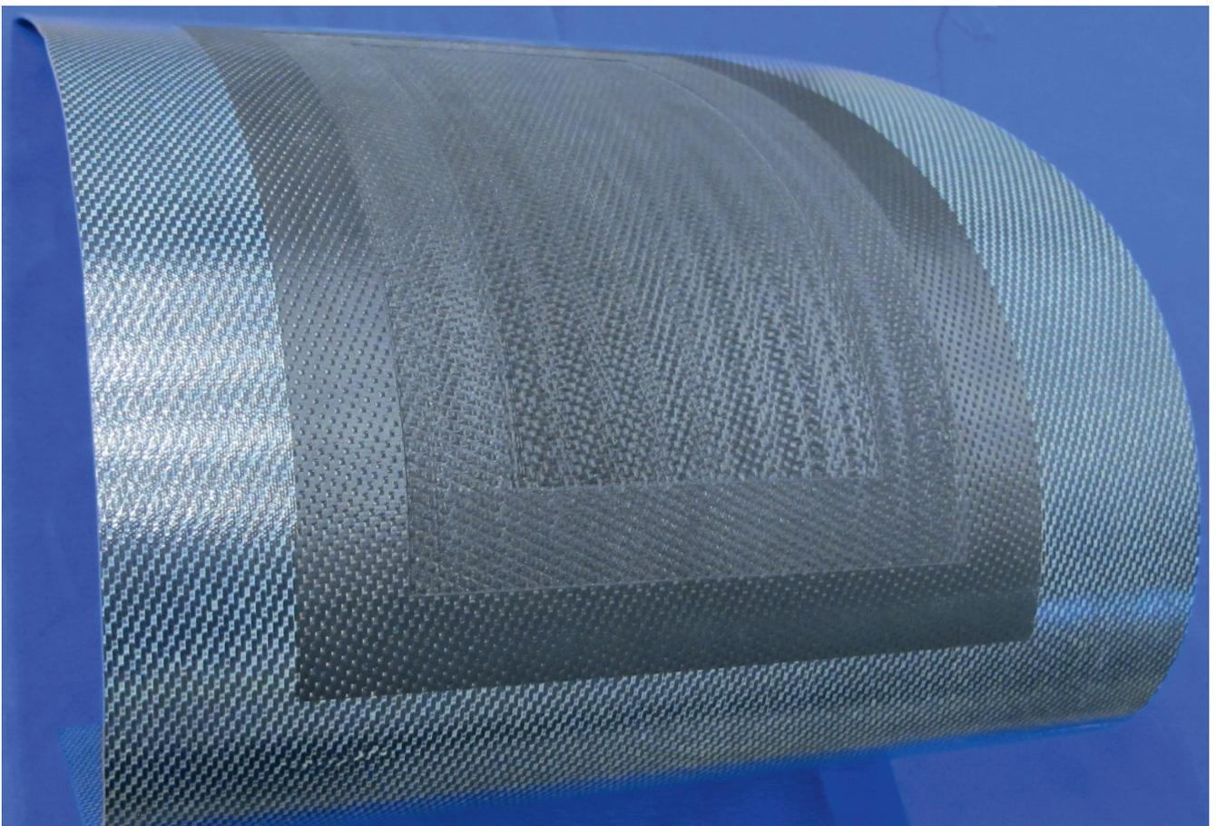
Stepped scarfing on slat demonstrator: scarfing is a challenging step in CFRP repair © LZH
