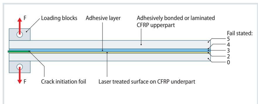
**Fig. 2.** Schematic principle of  $G_c$  coupon with highlighted positions of five fail-states
